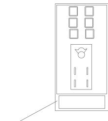
Accessible driver box for battery or controller
