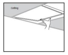
4.)Place the Backlit panel light into ceiling, then close the other side ceiling
