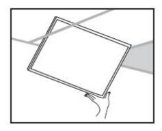
3.) Insert the Backlit panel light on the ceiling
