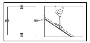
1.) Put on bracket / clip at the fitting with screws.
