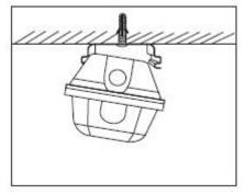
2.) Insert the fitting into the bracket at the ceiling
