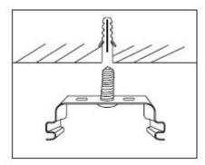
1.) Insert the wall plug into the ceiling, 2 sides
