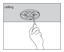
1.) Fix the mounting bracket to the ceiling with 2 screws.
