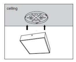
2.) Join the downlight to mouting bracket fixed with screw
