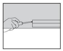
1.) Loose the 2 screws, left and right from the mounting bracket
