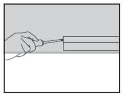
1.) Loose the 2 screws, left and right from the mounting bracket
