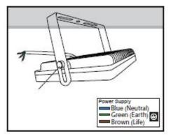
3.) Connecting the power supply wiring according to Blue, Green & Brown.
