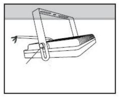
2.) Adjust the bracket to 90", then tight the screw at both side.
