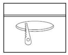
1.) Cut the ceiling hole according to the cutout size
