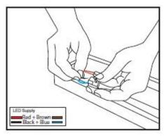
3.) Connect the Black colour wire together with Blue wire and Red colour wire together with Brown wire.
