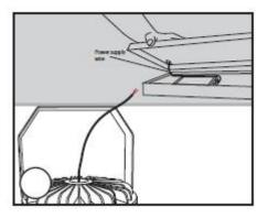
2.) Insert the LED Supply into the driver box
