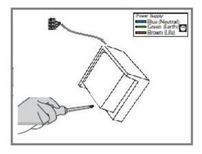
3.) Put on screw and fix it up on wall.
