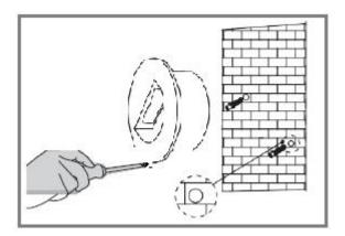
3.) Put on screw and fix it up on wall.
